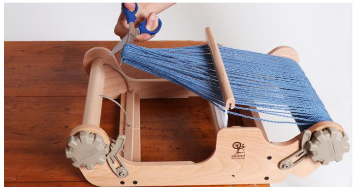
6. Stop winding once the yarn loops reach the front of the loom. Cut through the yarn loops. Unclamp the loom and follow the 'Learn to weave' booklet for threading the reed.
