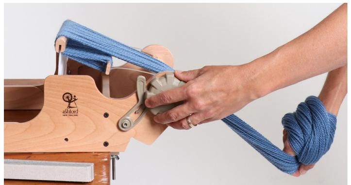
4. Stand at the back of the loom. Turn the back handle towards you allowing the threads to pass through your hand. Wind until the back warp stick goes around the roller once.
