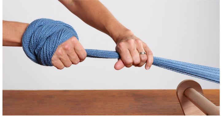
2. Twist the threads around your hand, maintaining an even firm tension, until you reach the front roller.
